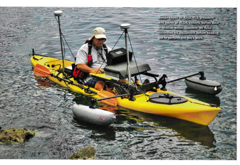
Compass systems, which are designed to provide a highly accurate GPS heading that takes into account the pitch, roll, and speed of vessels. To obtain accurate depth data, the team added a Teledyne Odom hydrographic echosounder.
