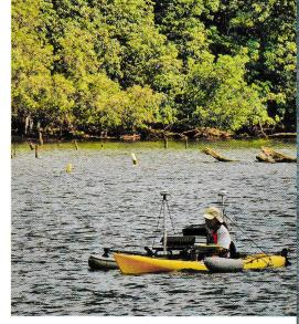
The kayak platform provides a low-maintenance, highly efficient surveying tool. Below: The main battery runs the electric kayak motor for a full day. An additional three-battery bank behind the operator (not shown) provides adequate power for the GPS and echosounder equipment.
